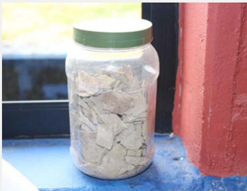
Figure 3.12: Desiccated lime found in water
